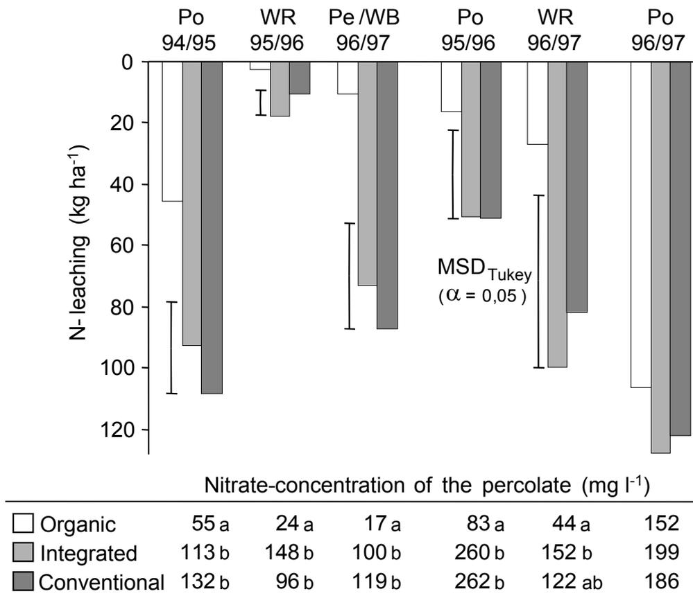
**Fig. 3.** Leached nitrate-N and mean nitrate concentration of soil water in 135 cm soil depth at the loamy sand site (Po - Potatoes; Wb/Wr – Winter barley/rye)
